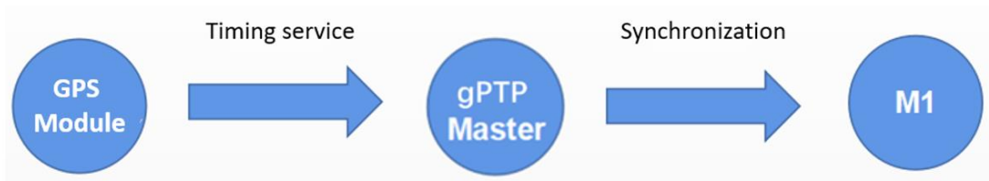
Figure 6: Topology of GPS Timing service synchronization
